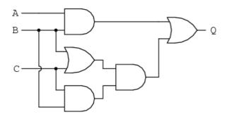
What will be the reduced form of the above circuit? (b) Differentiate between disjunction and conjunction.
