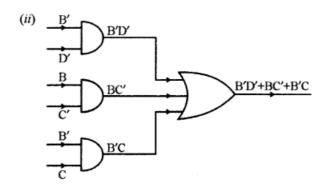
(ii) (a) From the logic circuit diagram given below, name the 3 output signals and finally derive the Boolean expression (F).
